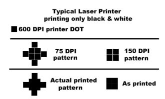
In the above diagram, the bottom row represents the shape and look of a single image pixel as printed. The 75 DPI pixel would be made up of 8 smaller printer pixels. In the 150 DPI example, 4 printer pixels would be used to create a 150 DPI image pixel. If the image being printed contains only black and white areas, then the highest printer resolution will yield the best result. This might include a line drawing or blueprint. So what about photographs?
