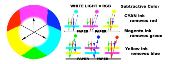
When two inks are used, they each remove their complimentary color leaving behind only one of the primary colors of light. Hence, cyan ink removes red, yellow ink removes blue, and only the color green is transmitted and reflected back to the viewer. If all three inks are used, then they effectively remove all wavelengths of light, and the result in no (zero) reflectance or black. When no ink is applied to an area the white paper reflects all wavelengths giving white.
