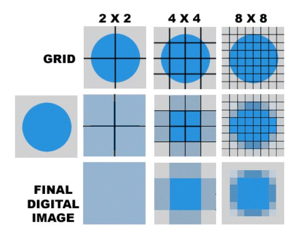
The top row represents the divisions that are used for camera sampling, the middle row shows the grid with the averaged colors for each pixel, and the final row shows the resultant digital image. The shape actually begins to appear in the 8 by 8 pixel image. More resolution (more pixels) will produce more detail in the digital image. More is better for image quality.
